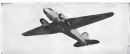
4. Practically every air traveler in the world has enjoyed the luxury of the Douglas DC-3. With two engines making out a total of 2100 h.p., it flies at a dependable 180 m.p.h. It usually carries 21 passengers and a crew of three.
